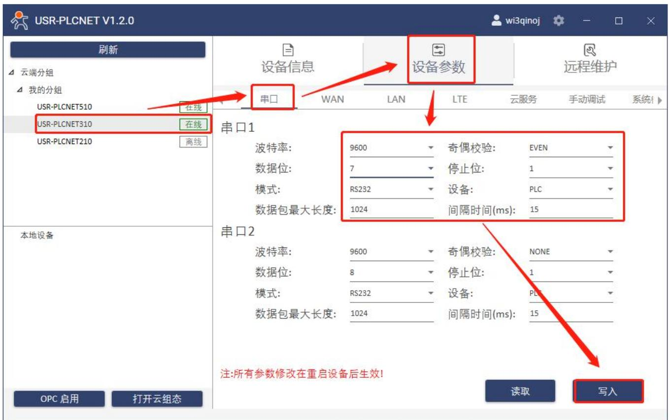
The screenshot shows the 'USR-PLCNET V1.2.0' software interface. On the left, a device list includes 'USR-PLCNET510' (在线), 'USR-PLCNET310' (在线), and 'USR-PLCNET210' (离线). The '设备参数' (Device Parameters) tab is selected, and the '串口' (Serial Port) sub-tab is active. The '串口1' (Serial Port 1) configuration table is highlighted with a red box:
